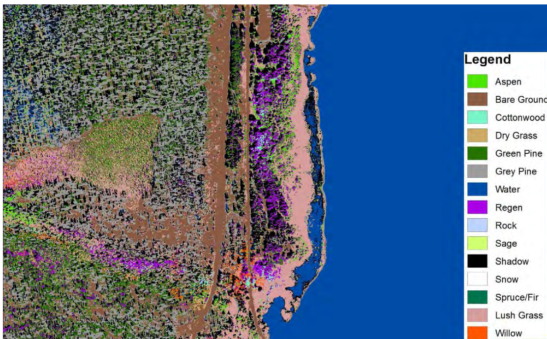
Figure 10: Example area from an early-stage land-cover model. We are building the classification layer at half-meter resolution, meaning that each pixel in the image represents a 0.5m x 0.5m area on the ground. The tree-level distinction between live and dead pines is apparent in the upper-left corner.
